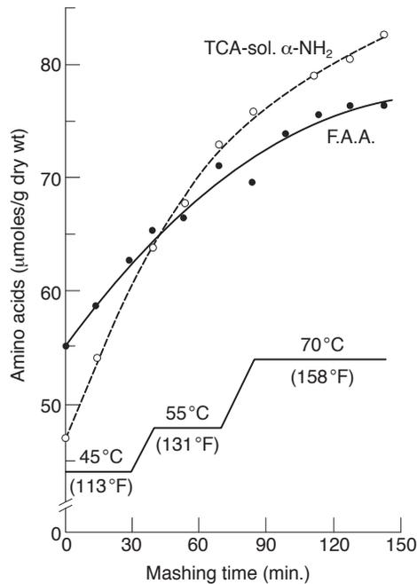
**Fig. 4.12** The formation of amino acids during a temperature-programmed mash (after Enari, 1974). The 'amino acids' were estimated in two different ways, which gave discordant results. Although amino acid liberation proceeded fastest at low temperatures it was still going on at the end of the mash at the highest temperature. (FAA, free amino acids; TCA sol- $\alpha$ -NH<sub>2</sub>, amino groups soluble in trichloroacetic acid.)
