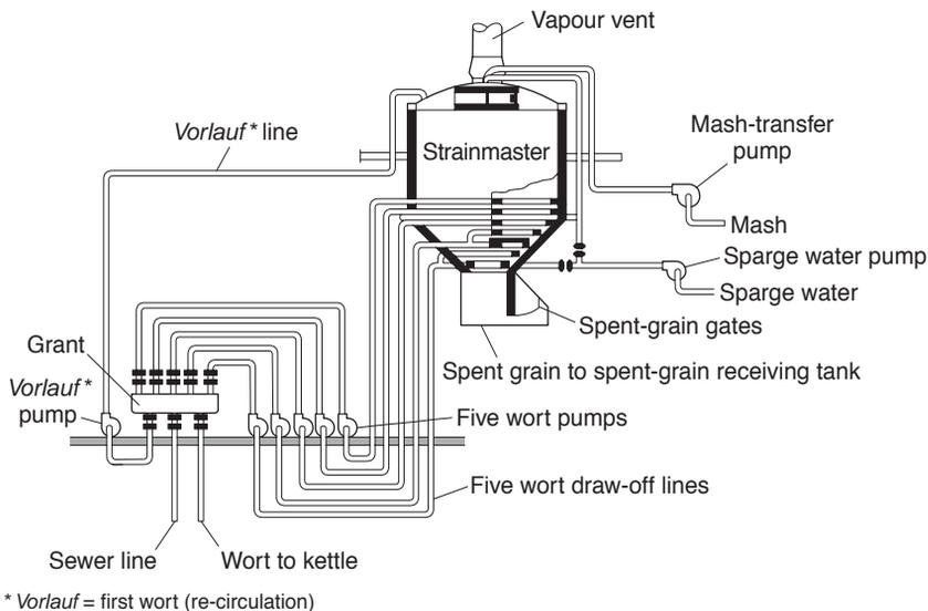
**Fig. 6.18** A Strainmaster lauter tun. The patent is owned by Anheuser-Busch (after Briggs *et al.*, 1981).
