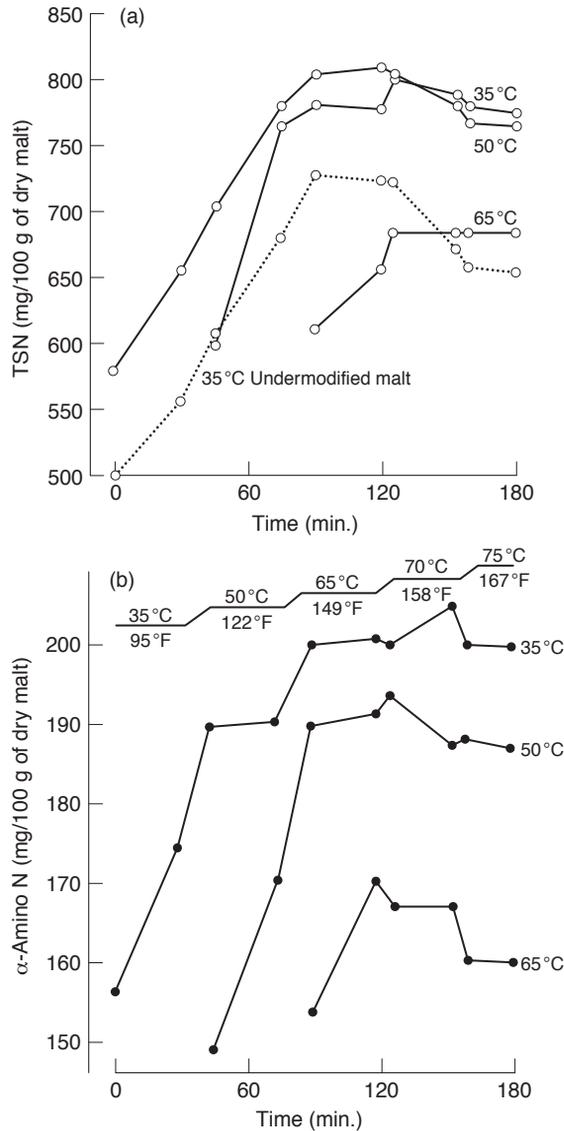
**Fig. 4.11** Increases in the levels of the (a) total soluble nitrogen and (b) the  $\alpha$ -amino nitrogen during temperature-programmed mashing. The different mashes were started at the temperatures shown and then the programme was completed (after Narziss, 1977). The discontinuous line in (a) shows the results obtained with a different, undermodified malt.
