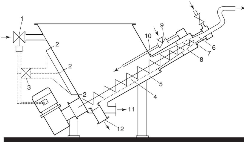
**Fig. 10.19** A hop separator (Hough *et al.*, 1982, courtesy of A. Ziemann, GmbH). 1. Valve; 2. Level control electrodes; 3. Level controller; 4. Helical screw conveyor; 5. Sieve/strainer; 6. Compression chamber, where the hops are squeezed; 7. Fasteners; 8. Wort receiver under the second strainer; 9. Three-way valve (wort return and sparge water); 10. Return pipe; 11. Wort discharge; 12. Clean-out valve. Spent hops are discharged at the top.
