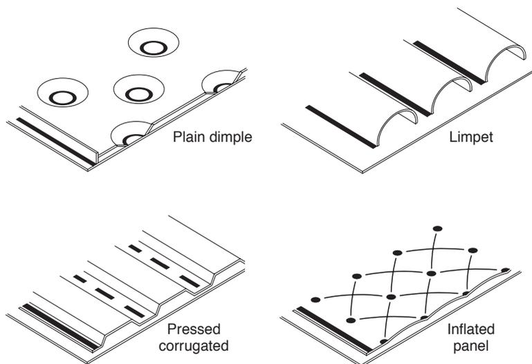
**Fig. 15.2** Designs of cooling jackets for dual-purpose fermenting vessels: plain jacket, not usually used because it requires thick vessel construction to resist external pressures; limpet, provides a flow-path for coolant, but again relatively heavy; pressed corrugated, lighter construction than limpet and widely used for secondary refrigerant systems; inflated panel, low volume and suited to primary refrigerant systems acting as an evaporator (Barnes, 2001).
