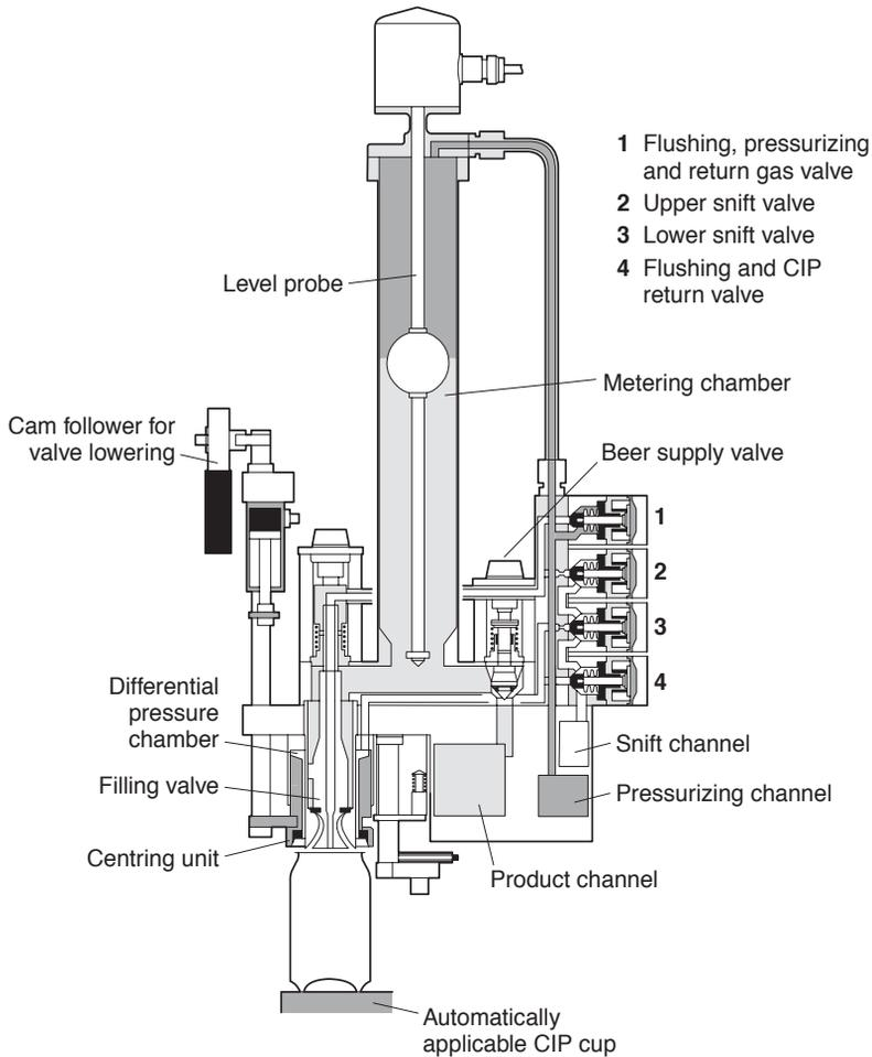
**Fig. 21.12** Can filling valve (by courtesy of Krones).
