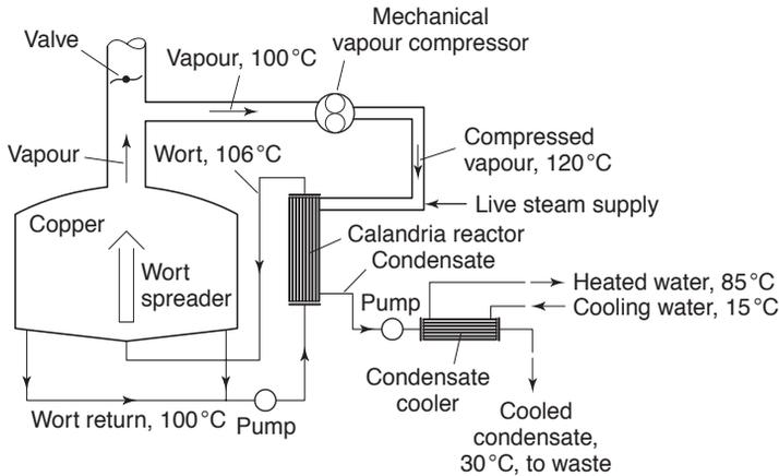
**Fig. 10.14** Outline of a mechanical vapour recompression (MVR) system (after Fortuin, 1995).
