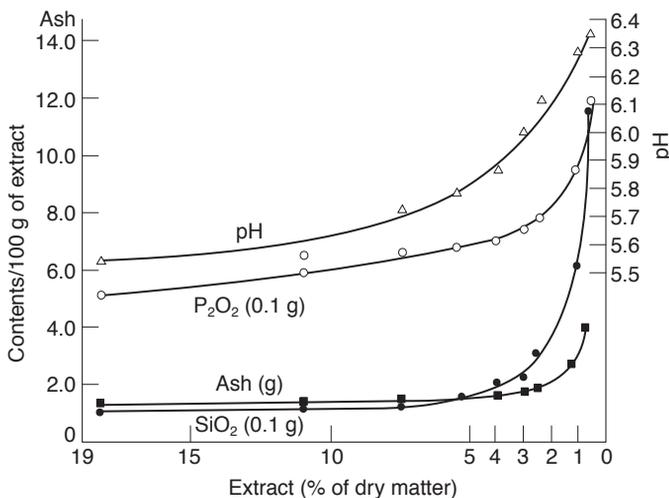
**Fig. 4.16** Alterations in wort pH, phosphate content (as P<sub>2</sub>O<sub>5</sub>), ash content and silica content during wort separation and sparging (after Schild, 1936; see also Fig. 4.15).
