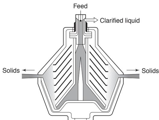
**Fig. 15.9** Self-cleaning clarifier centrifuge (Hough, *et al.*, 1982).
