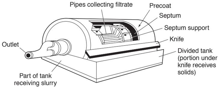
**Fig. 15.11** Rotary vacuum filter (Hough *et al.*, 1982).
