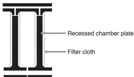
**Fig. 6.21** Two recessed chamber plates, seen in vertical section (after Nguyen, 1996). The space between the cloths is the mash chamber. The wort is collected in the spaces between the cloths and the plate partitions.
