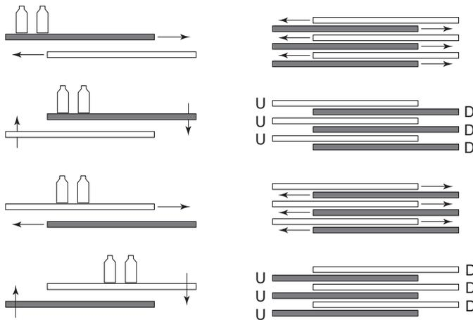
**Fig. 21.10** Walking beam principle for moving bottles through a tunnel pasteurizer. Left-hand sequence represents side elevations showing successive movements of shaded grid beams in relation to unshaded grid. Right-hand sequence represents corresponding plan views (D indicates downward movement and U upward movement), (Coleman, 1976 and Hough *et al.*, 1982).
