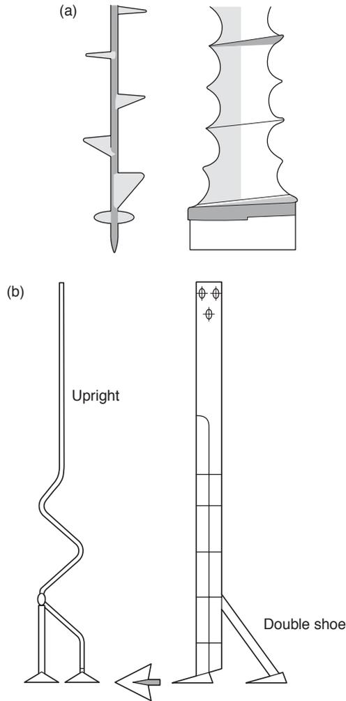
**Fig. 6.15** A lauter tun knife equipped with ‘winglets’ to lift the mash (after Andrews and Wilkinson, 1996). Note the plastic base to the ‘shoe’ which minimizes the risk of damage to the false bottom of the tun. (b) A pattern of double shoe lauter tun knife with a ‘zig-zag’, chevron-shaped blade (Lenz, 1989).
