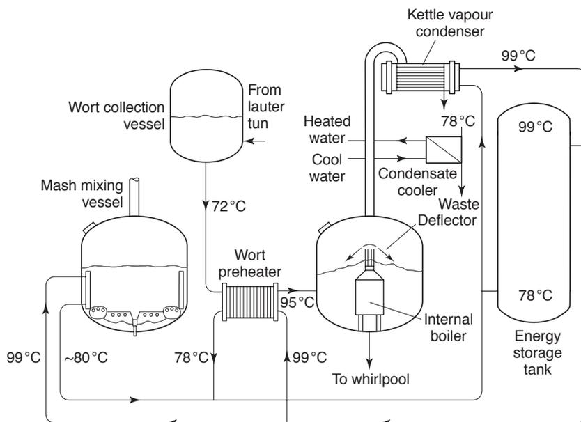
**Fig. 10.13** An arrangement where vapour from a kettle is condensed and heat recovered in hot water is stored in a temperature gradient tank and is partly used to heat the wall jacket of a mash mixing vessel and the wort from the lauter tun, before it enters the copper (after Herrmann, 1998b).
