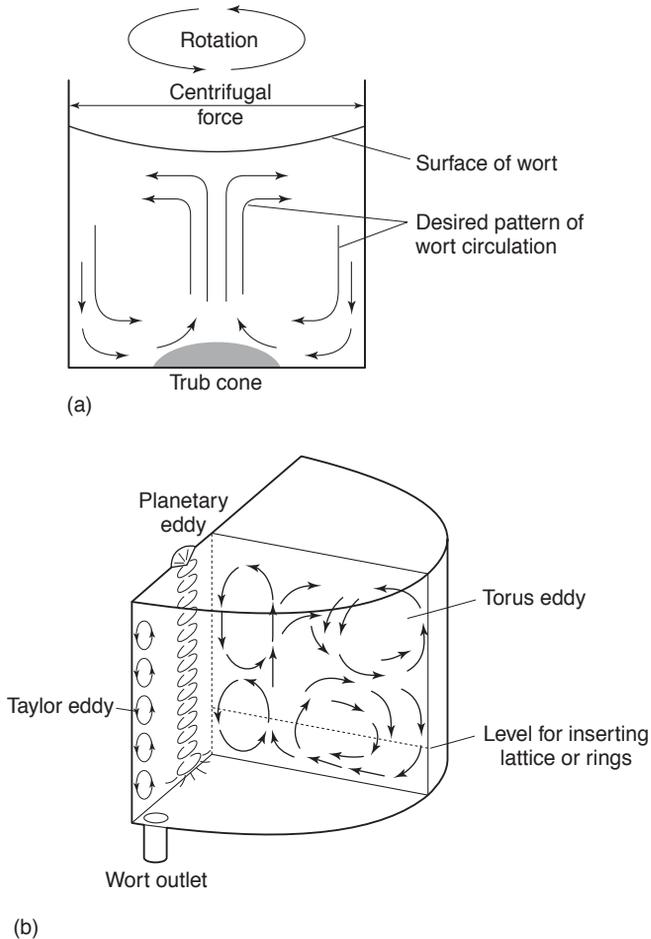
**Fig. 10.21** Currents in whirlpool tanks. (a) The ideal flow pattern in a whirlpool. (b) Undesirable eddy currents that can occur and which interfere with trub separation. The most troublesome are the torus eddies, which may be checked by the insertion of a lattice or rings at the level indicated (after Denk, 1991).
