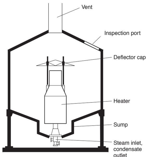
**Fig. 10.8** A diagram of a copper having an internal heater, mounted over and extending partly into, a 'cup' or 'sump'. The extra depth permits the heater to be larger than would otherwise be the case, and so it has a large heat transfer surface (after Michel, 1991).
