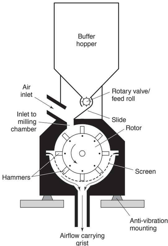
**Fig. 5.7** The layout of a type of hammer mill (various sources).
