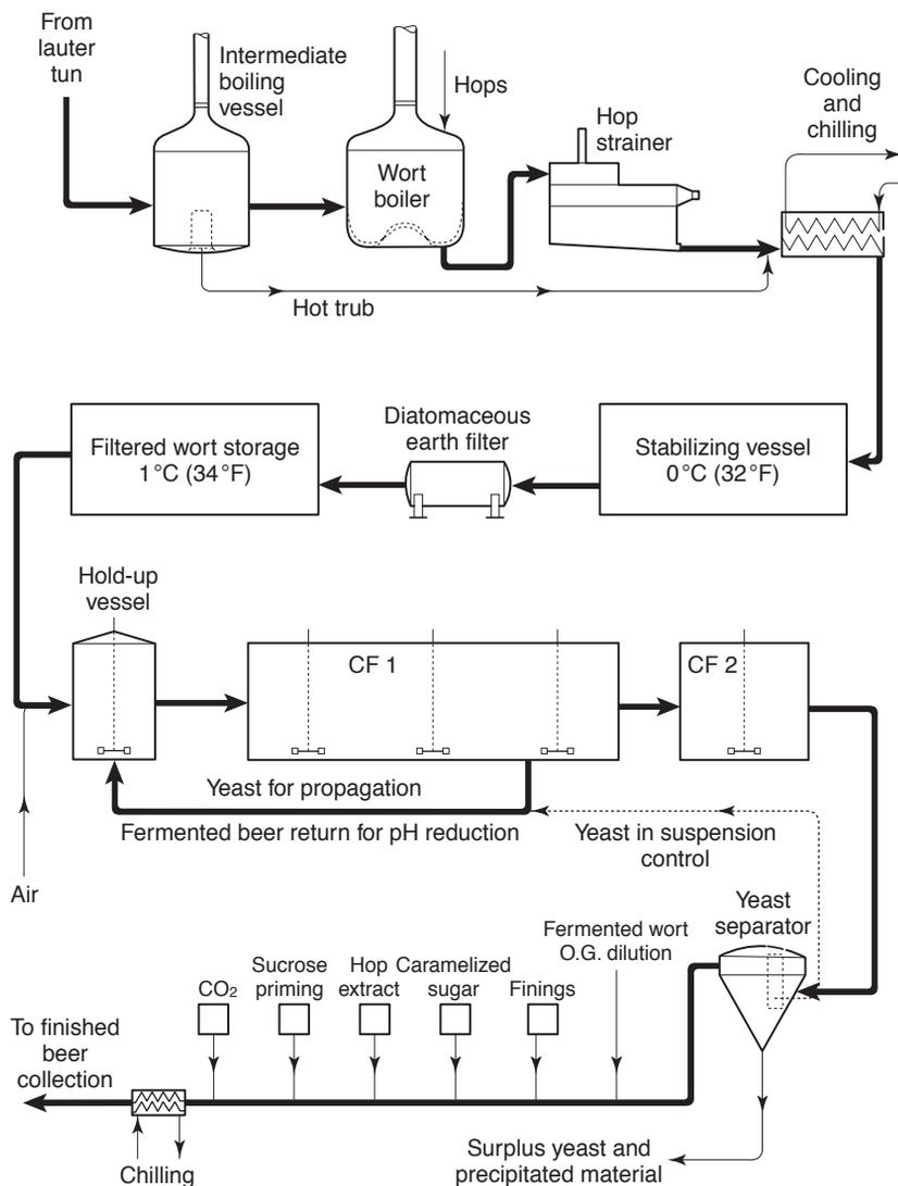
**Fig. 14.12** New Zealand system of continuous fermentation, (CF1) continuous fermenter 1, (CF2) continuous fermenter 2 (Coutts, 1957, 1958).
