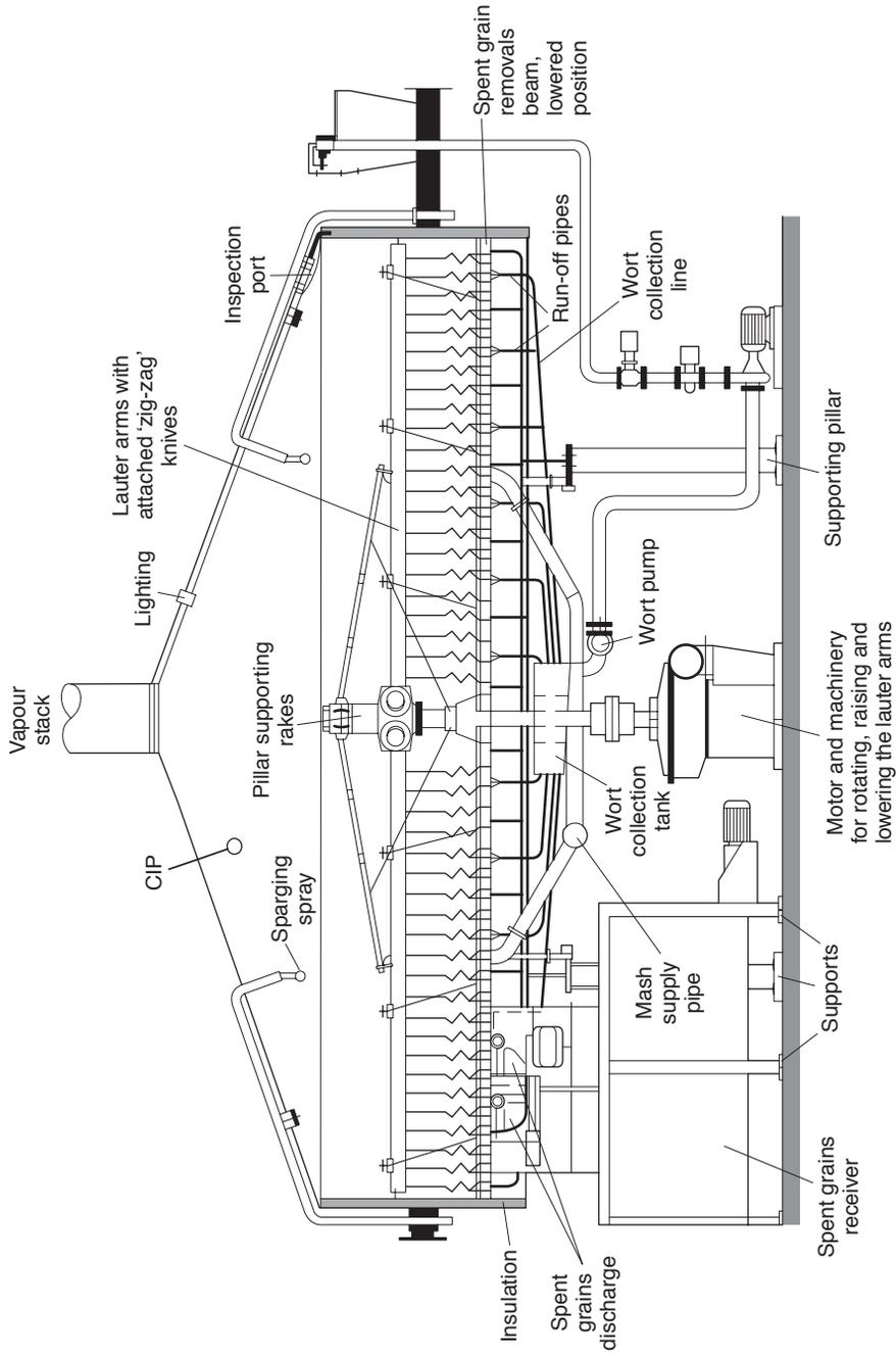
**Fig. 6.13** A section of a modern lauter tun equipped with fixed sparging nozzles and zig-zag, chevron-shaped knives, the outer ones of which are the double-shoe type (after Herrmann *et al.*, 1990).
