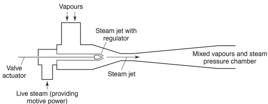
**Fig. 10.15** The principle of a steam-jet vapour compressor. A regulated jet of live steam sucks vapours into the nozzle. As the cross-sectional area of the tubing widens the stream of mixed steam and vapour slows down and the pressure rises, e.g., to 1.2–1.7 bar (104.8–115.2 °C; approx. 221–239 °F).
