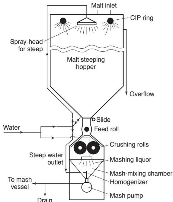
**Fig. 5.9** A mill using steep conditioning (various sources).
