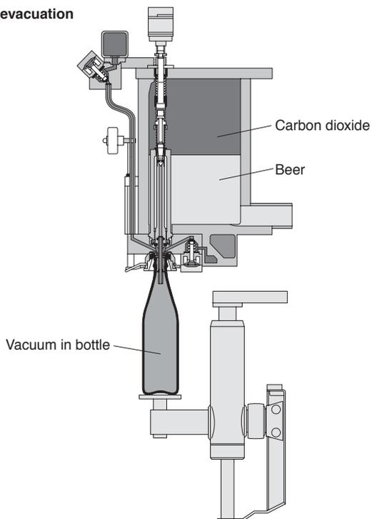
**Fig. 21.6** (c) 2nd evacuation (vacuum in bottle) (by courtesy of Kronen).
