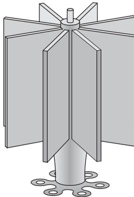
**Fig. 10.5** A 'star' steam-heater, designed to have a large surface area while remaining compact, and be suitable for mounting in the base of a copper (Hough *et al.*, 1982).
