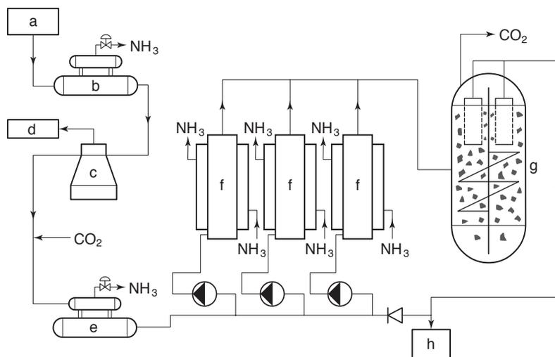
**Fig. 15.18** Ice beer plant, Labatt/Niro; (a) route from fermentation, (b) dropping cooler, (c) centrifuge, (d) yeast, (e) beer cooler, (f) heat exchanger, (g) recrystallizer, (h) route to conditioning. (Kunze, 1999).
