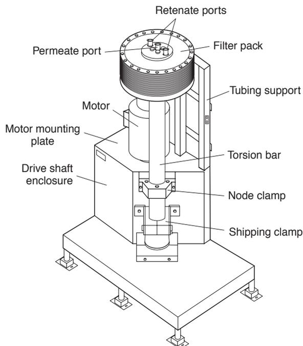
**Fig. 15.12** Vibrating membrane filter (Chalmers, and Haughney, 1998).
