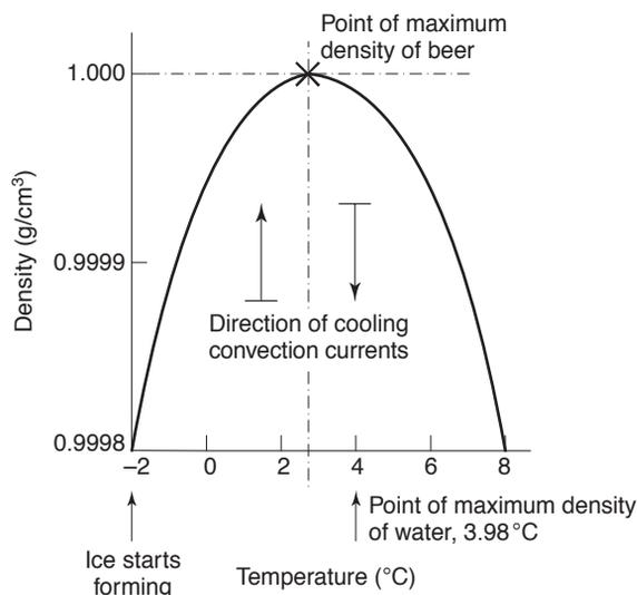
**Fig. 14.4** Change in density of fermenting beer with change in temperature (Barnes, 2001).
