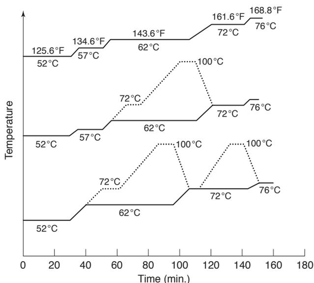
**Fig. 4.6** The temperature programmes of three mashes that yield very similar worts (after Hug and Pfenninger, 1979). The uppermost scheme is for a temperature-programmed infusion mash while the central scheme is for a single-decoction mash and the lowest is for a double-decoction mash.
