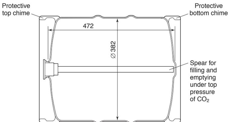
**Fig. 21.13** Vertical section of a 50l beer keg, height 472 mm; diameter 382 mm (by courtesy of Alumasc Ltd).
