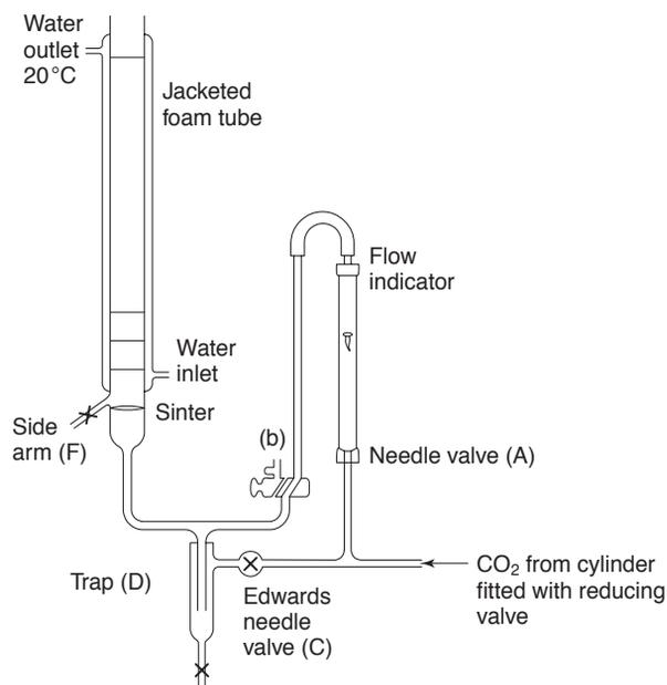
**Fig. 19.6** Rudin head retention apparatus (Institute of Brewing, Methods of Analysis, 1997).
