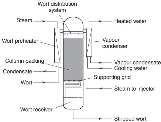
**Fig. 10.12** A steam stripper for removing volatiles from wort (after Bonachelli *et al.*, 2001; Seldeslachts *et al.*, 1997).
