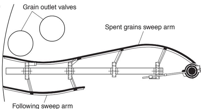
**Fig. 6.16** (a) A lauter tun with the grain discharge plough bar in the raised (rest) and lowered (graining-out) working positions (after Barnes, 2000). (b) A plan view of another pattern of grain plough with a trailing, second sweep arm (after Herrmann *et al.*, 1990).
