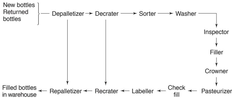
**Fig. 21.1** Arrangement of equipment in a bottling hall (Hough *et al.*, 1982).
