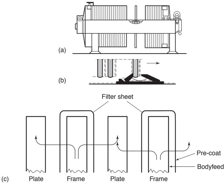
**Fig. 15.15** Plate and frame filter; (a) side view, (b) automatic mechanism for moving individual plates for opening and closing, (c) arrangement of plates and frames and the flow of beer. (Courtesy of Alfa-Laval Ltd.).
