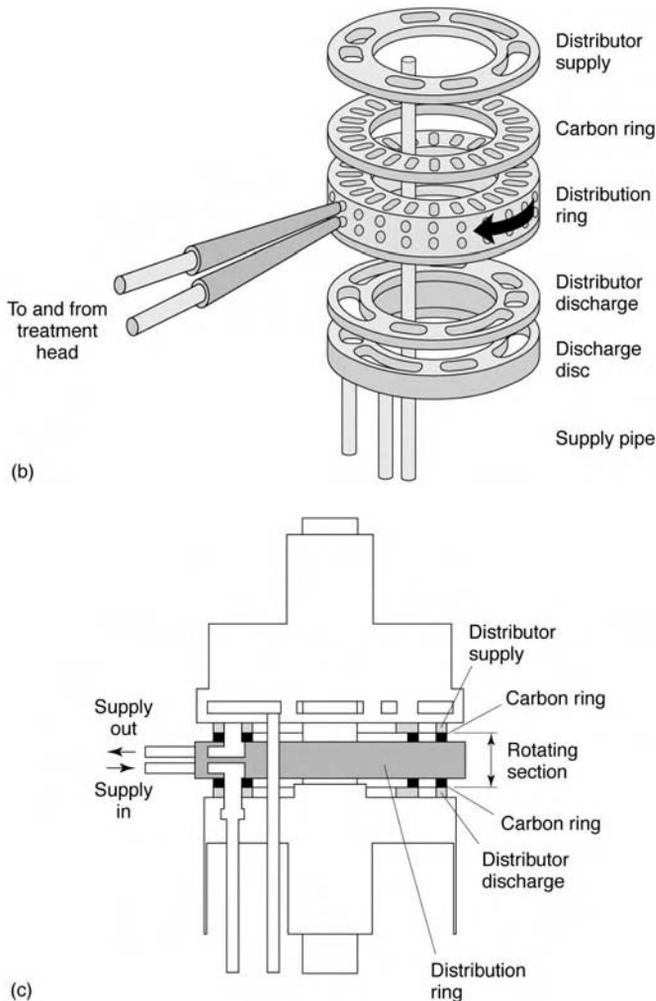
**Fig. 21.16(b) and (c)** Central distributor of the rotary keg racking machine shown as (b) a schematic block diagram and (c) in vertical section. Each seal for the supply and return of services comprises two discs: a carbon ring and a metal distributor ring. When the holes of the two rings in the rotating section are aligned liquid will flow to the head (Courtesy of KHS Till and Eaton, 2002).
