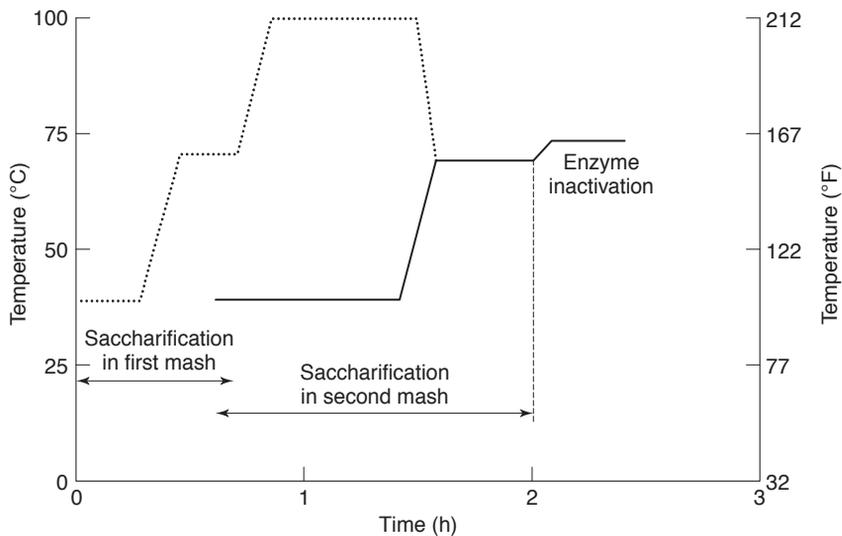
**Fig. 4.5** A scheme of the temperatures found in a double-mash programme using a grits cooker (after Hind, 1950). ..... the temperature of the adjuncts/grits mash in the cereal cooker. — the temperature in the malt mash and in the combined mash during and after mixing.
