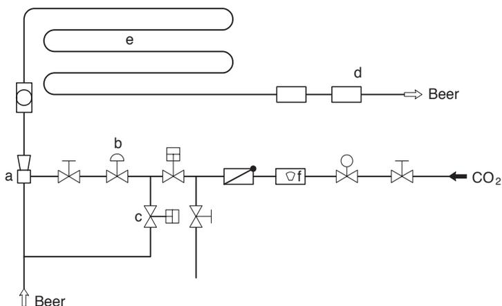
**Fig. 15.7** Carbonation unit; (a) venturi nozzle, (b) carbon dioxide control valve, (c) CIP valve, (d) carbon dioxide sensor, (e) carbon dioxide dissolving area, (f) carbon dioxide measuring device (Kunze, 1999).
