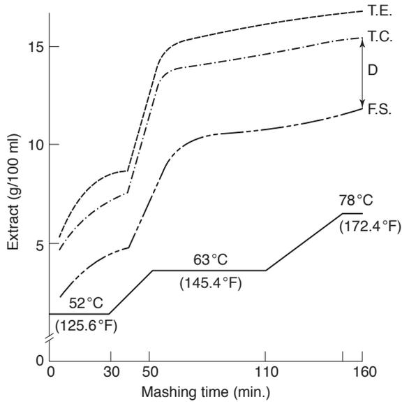
**Fig. 4.10** Changes in the yield of total extract (TE), the yield of total carbohydrate (TC), the fermentable sugars (FS) and the unfermentable dextrins (D) during a temperature-programmed mash (after Enevoldsen, 1974).
