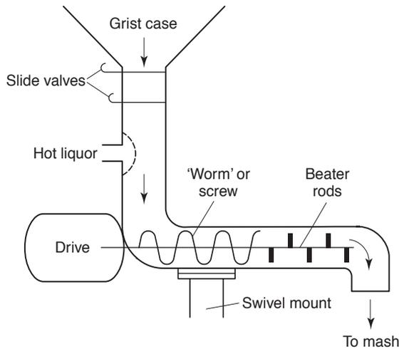
**Fig. 6.2** Steel's mashing machine, used in traditional British infusion mashing. In more modern versions the rate of grist flow is regulated mechanically and the slide valves prevent steam from the mash travelling into the grist case.
