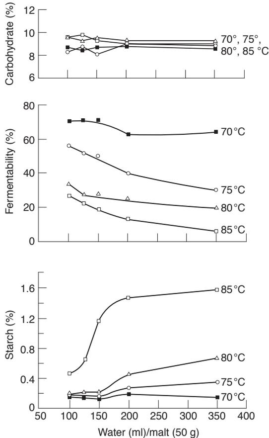
**Fig. 4.13** The influences of mash thickness and mash temperature, during 1 h. isothermal mashing, on (upper) the yield of carbohydrate in the wort, (middle) the fermentability of the wort and (lower) the starch present in the wort (after Muller, 1991).
