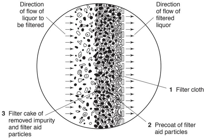
**Fig. 15.14** Principles of kieselguhr filtration (Hough *et al.*, 1982).
