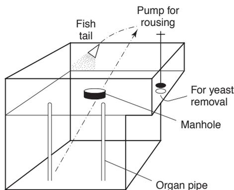
**Fig. 14.8** Yorkshire square fermenting vessel (Hough *et al.*, 1982).
