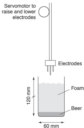
**Fig. 19.7** NIBEM foam stability apparatus (after Klopper, 1973).
