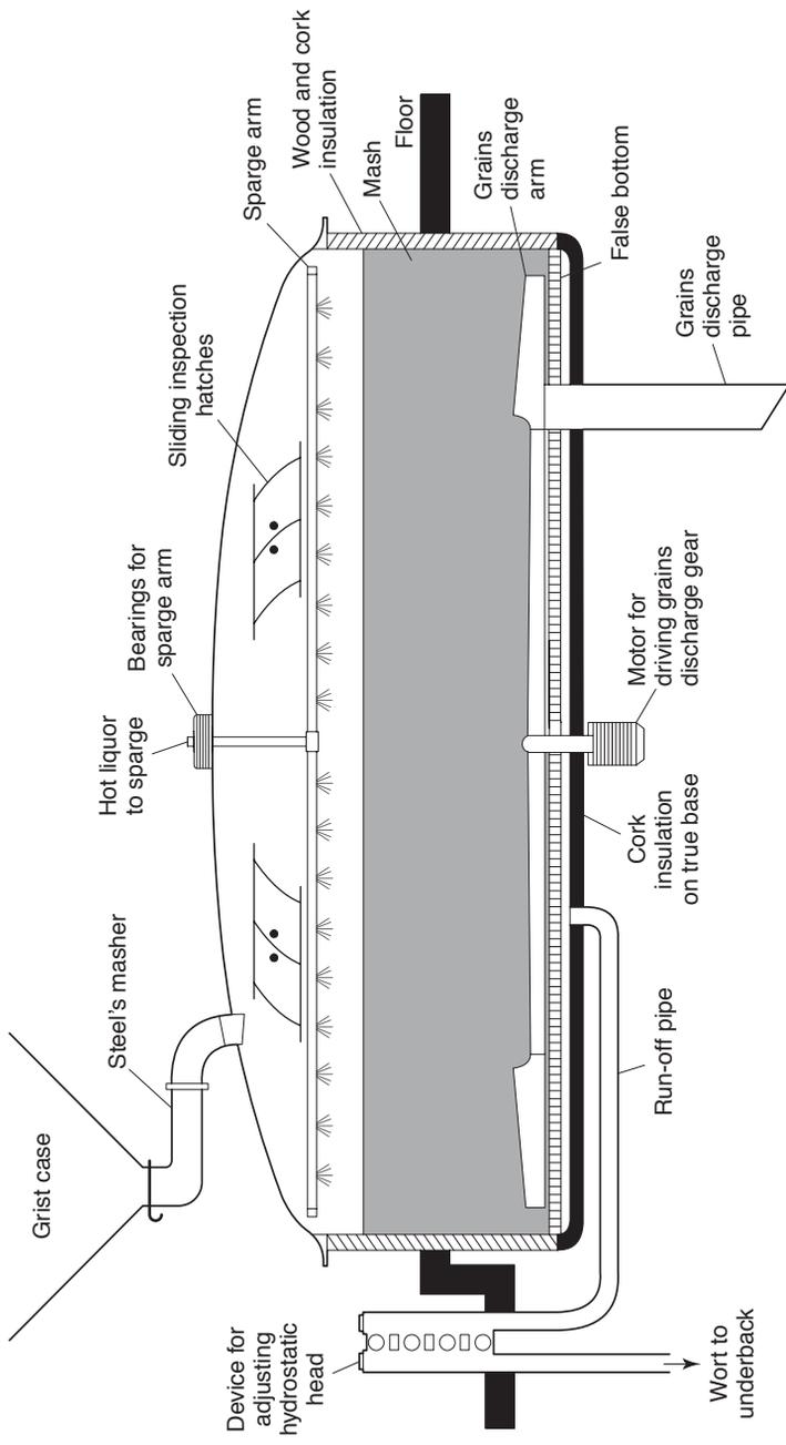
**Fig. 6.7** A current pattern of mash tun (after Briggs *et al.*, 1981).
