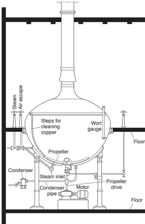
**Fig. 10.2** An old pattern of copper having a rounded base and heated by a symmetrical, external steam jacket (after Hind, 1940).
