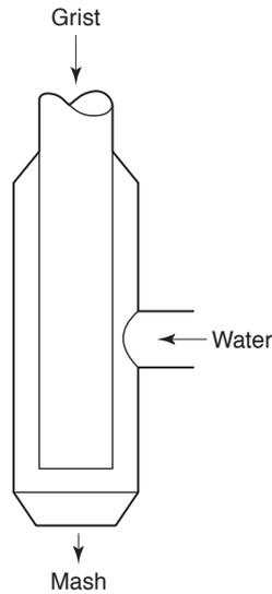
**Fig. 6.5** A vortex mash mixer (after Rehberger and Luther, 1994). The grist falls into a swirling tube of liquor from that tangentially injected into the outer chamber. With these, and other pre-hydrators, it is desirable to have a mixing chamber through which the grist must pass before it leaves the unit.
