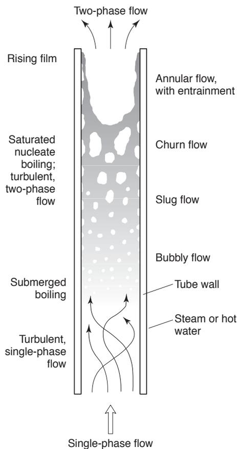
**Fig. 10.1** Diagram of the stages of boiling in wort rising up a steam- or water-heated tube (after Wilkinson, 1991a, b). As the wort rises so boiling becomes more vigorous, the flow becomes ‘two-phase’ as steam vapour bubbles appear and come to occupy an increasing proportion of the volume.
