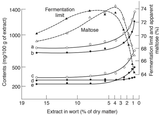
**Fig. 4.15** Changes in the composition of sweet wort during run-off and sparging (after Schild, 1936).  $\blacktriangle$  ---  $\blacktriangle$  fermentation limit;  $\triangle$  ---  $\triangle$  apparent maltose; (a) total soluble nitrogen; (b) permanently soluble nitrogen; (c) soluble nitrogen not precipitated by phosphotungstic acid; (d) formol nitrogen; (e) nitrogen not precipitated by tannic acid (see also Fig. 4.16).
