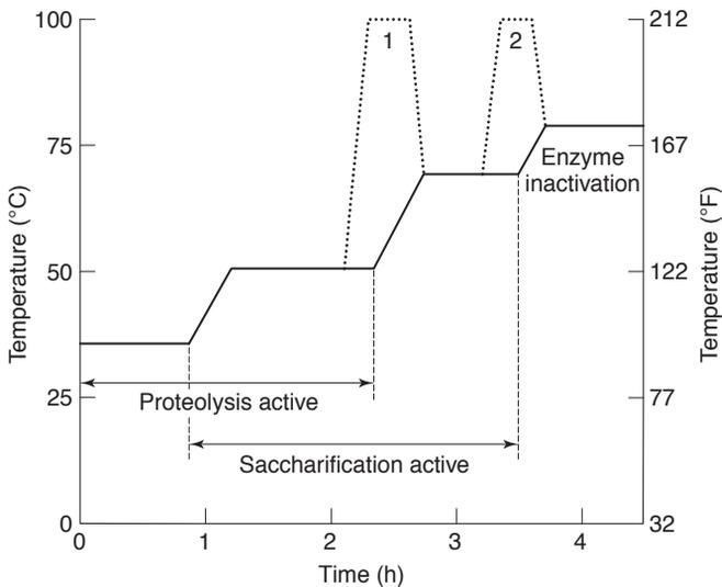
**Fig. 4.3** A temperature scheme for a typical two-decoction mashing programme (after Hind, 1950). The key is in Fig. 4.2. About a quarter of the mash is used in each decoction. Process duration, four and a half hours.
