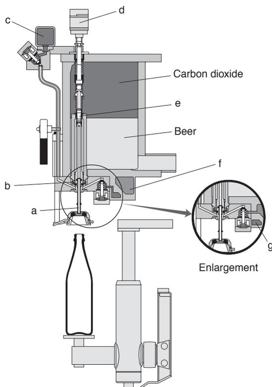
**Fig. 21.5** Bottle filling, section view; basic position before the bottle is lifted onto the filling head (air in bottle); a, vent tube; b, siphon type gas lock; c, correction channel; d, control cylinder for liquid valve and pressurizing; e, gas needle; f, vacuum/CIP channel; g, snift channel (by courtesy of Kronen).
