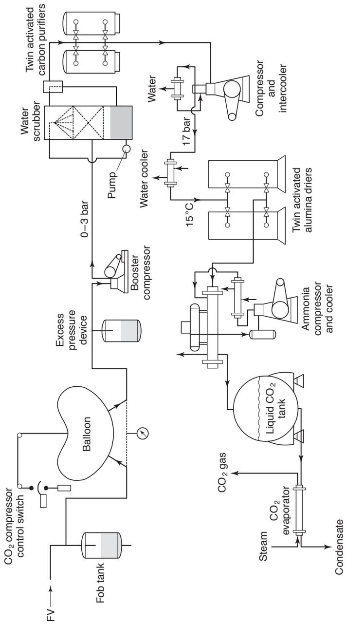
**Fig. 15.8** Equipment for collecting, purifying, storing, and releasing carbon dioxide (Hough *et al.*, 1982).
