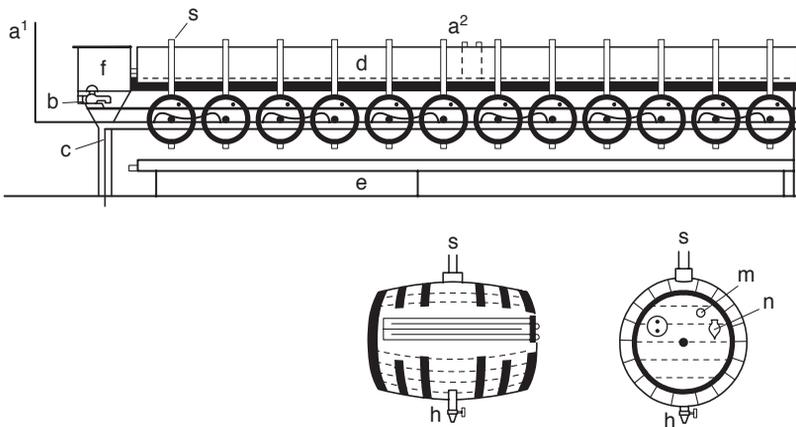
**Fig. 14.9** Burton Union fermentation system ( $a^1$ ) attemperator water (beer); ( $a^2$ ) attemperator water (yeast); (b) side rod; (c) waste water; (d) top trough; (e) bottom trough; (f) feeder; (s) swan-necks; (h) bottom tap; (m) side tap; (n) sample tap (Hough *et al.*, 1982).
