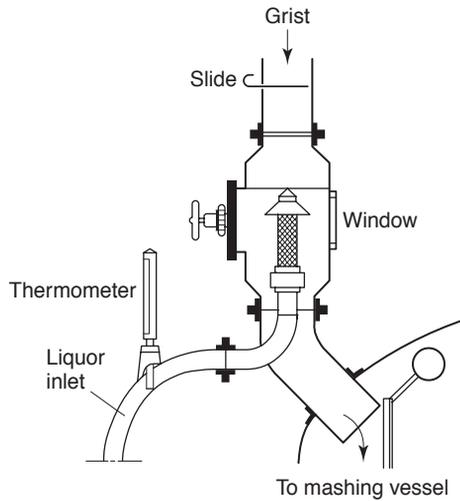
**Fig. 6.3** Premasher or Maitland grist hydrator, of a traditional mainland European type, used in conjunction with decoction mashing (after Narziss, 1992). Note that the grist falls past a perforated tube, which delivers the mashing liquor. The mixture pushes open a counter-balanced door and falls into the vessel.
