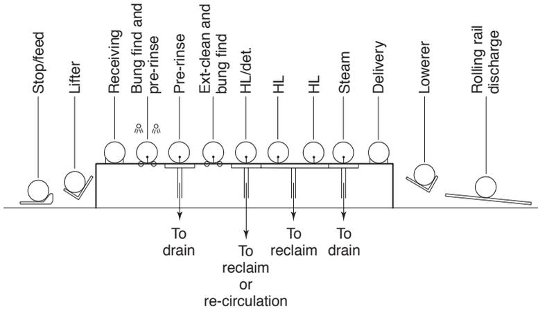
**Fig. 21.19** Internal cask washing equipment: nine station chain machine with moving centre beam; HL, hot liquor (water); det, detergent applied to outside of cask (not used in all installations) (by courtesy of Porter Lancastrian Ltd.).
