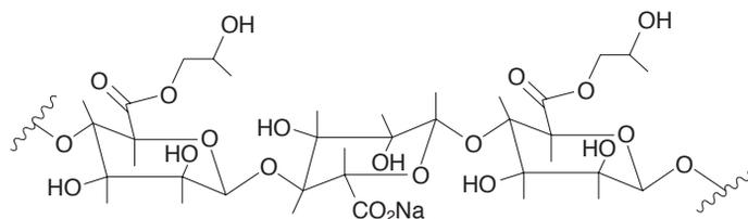
**Fig. 19.9** Idealized structure of propylene glycol alginate (Baxter and Hughes, 2001, Fig. 2.5).
