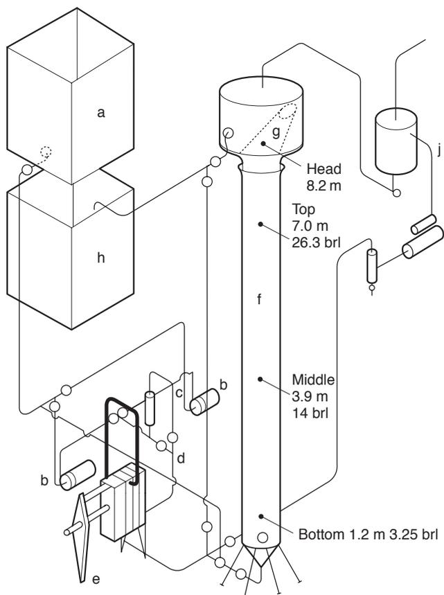
**Fig. 14.11** Continuous tower fermenter; (a) wort collection; (b) impeller pump; (c) flow meter; (d) control valve; (e) flash pasteurizer; (f) tower; (g) yeast separator; (h) beer receiver; (j) CO<sub>2</sub> collecting vessel (after Hough *et al.*, 1982).
