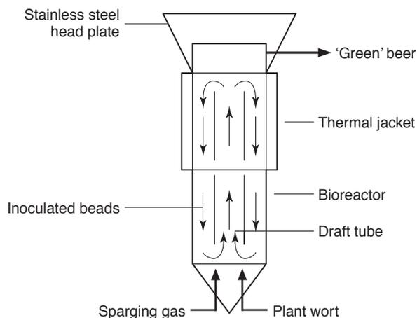
**Fig. 14.13** Gas lift draft tube bioreactor (Mensour *et al.*, 1997).
