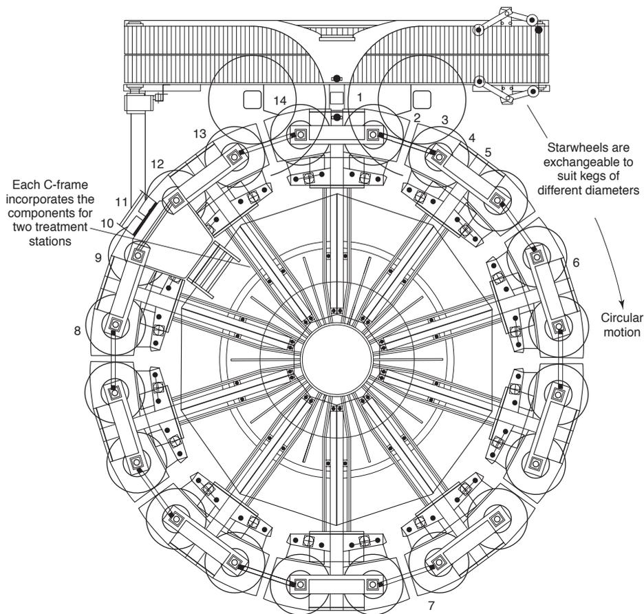
**Fig. 21.16(a)** A rotary keg racking machine shown in plan from the top. Kegs move around the central core at the series of stations which comprise: 1 cylinder down; 2 leak test; 3 rinse head; 4 blow out head; 5 pressure test; 6 counter-pressure; 7 fill; 8 disconnect; 9 rinse head; 10 pressure relief; 11 cylinder up; 12 close keg; 13 release keg clamp; 14 discharge keg (Eaton, 2002 and courtesy of KHS Till).
