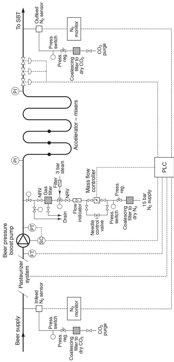
**Fig. 21.17** Flowsheet for the 'Nitroset' beer nitrogenation system: FT flow transmitter; SC speed controller; PT pressure transmitter; PI pressure indicator; NRV non-return valve; PLC programmable logic controller; SBT sterile beer tank (Lindsay *et al.*, 1995).
