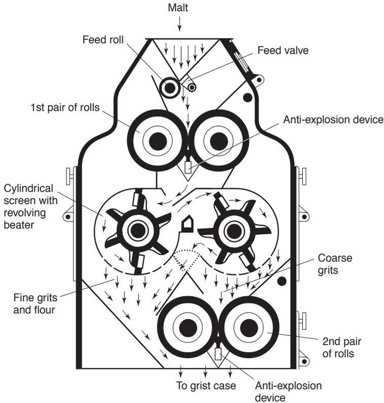
**Fig. 5.4** A four-roll mill using cylindrical screens to fractionate the grist from the first pair of rolls and to direct the coarse grits to the second pair of rolls (after Hind, 1950). Similar results are obtained in mills with oscillating, flat-bed screens.
