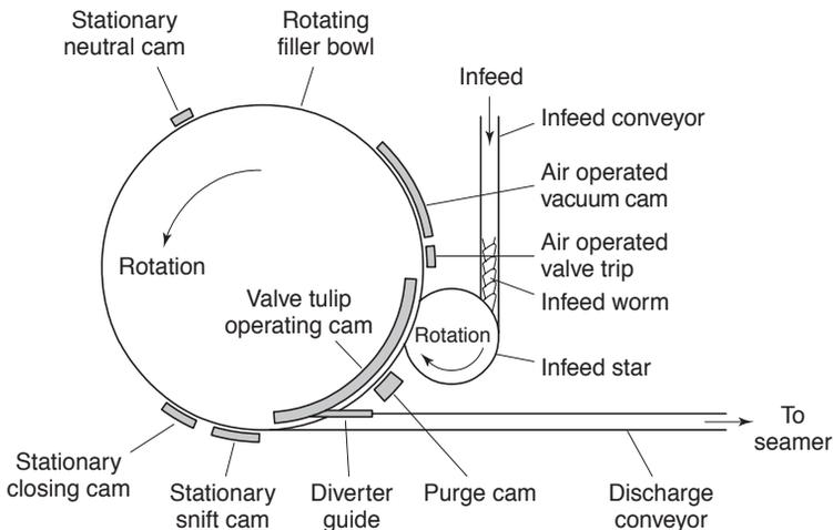
**Fig. 21.11** Can filling, schematic. Cans are fed to the infeed star, which places them on to the filler bowl platforms, one can beneath each filling valve. The can filling sequence then operates; as the bowl rotates, cams remove air from the can, charge with gas, fill with beer, close the valve and remove residual gas. (Heins and Heuer, 1997).
