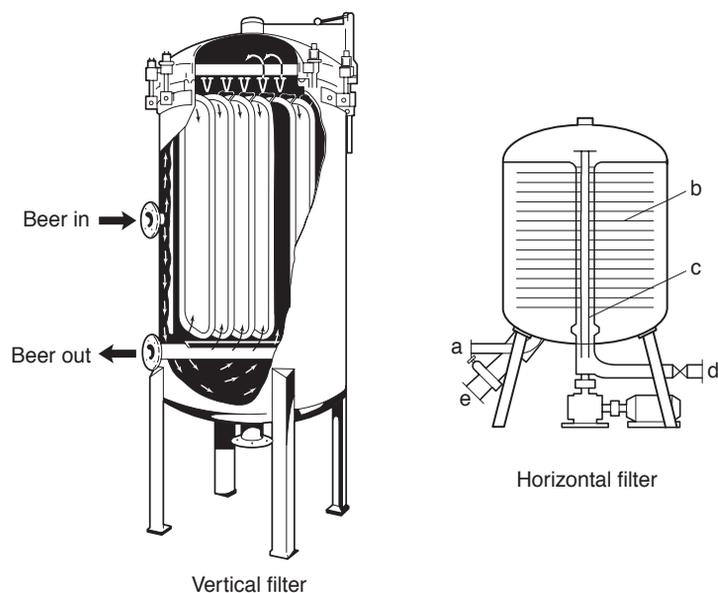
**Fig. 15.16** Vertical and horizontal leaf filters; horizontal filter: (a) beer inlet, (b) filter support, (c) perforated shaft, (d) filtered beer outlet, (e) sediment outlet (Courtesy of Alfa-Laval Ltd.).
