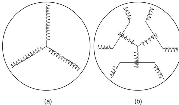
**Fig. 6.17** Possible arrangements of knives on the rotating arms in (a) a small lauter tun and (b) a large lauter tun. The knives rotate clockwise and are so spaced along the bars that they track between the slots made by the knives that precede them (Andrews and Wilkinson, 1996).
