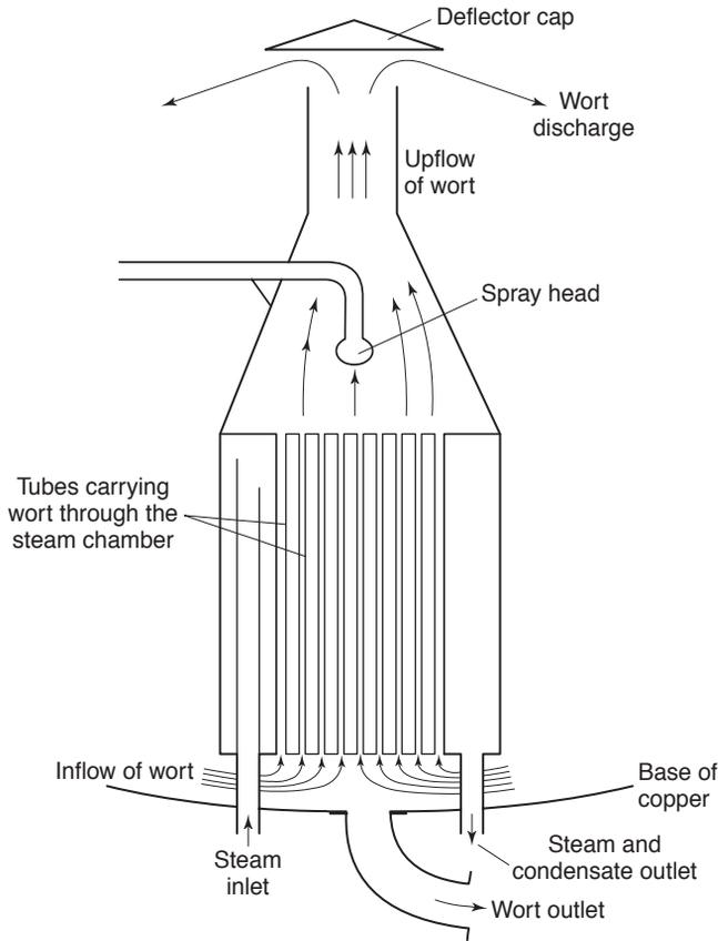
**Fig. 10.7** An internal heater and ‘fountain’ for coppers in which the wort moves up the steam-heated tubes by convection, its flow is constricted, then it emerges from beneath the wort level and strikes the deflector plate which directs it down onto the wort surface (Various sources).
