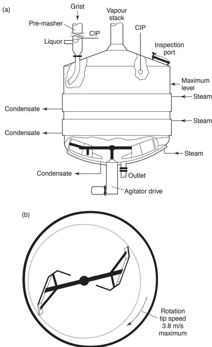
**Fig. 6.11** (a) A section of modern mash-mixing vessel. Note the inclined base (after Wilkinson and Andrews, 1996). (b) A plan view of the interior of the base of a mash-mixing vessel, showing the offset stirrer.
