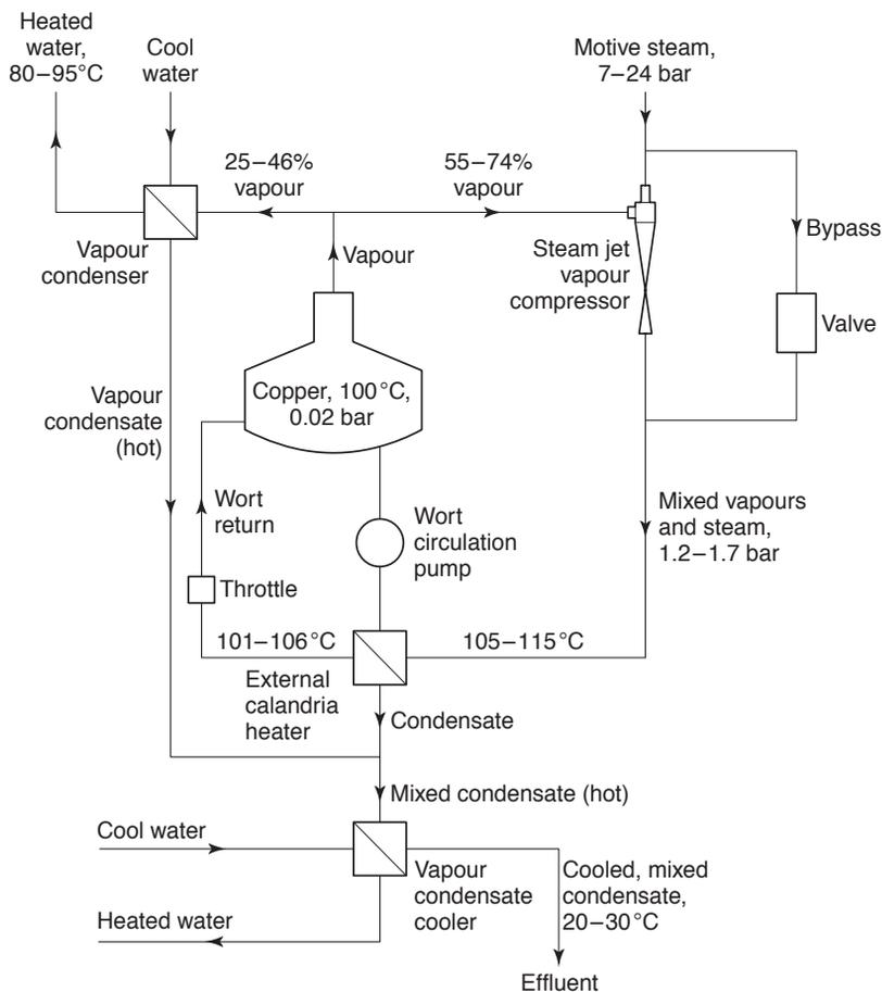
**Fig. 10.16** A thermal vapour recompression (TVR) system (after Fohr and Meyer-Pittroff, 1998). The wort is boiled, under pressure, by the compressed mixture of vapour and steam from the steam jet vapour compressor. Vapour from the copper that is not compressed is condensed and used to heat water in the process. Mixed condensates from the vapour condenser and the heater are cooled and sent to waste. Hot water is also obtained from this operation.
