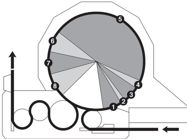
**Fig. 21.4** Bottle filling, plan view: 1, 1st evacuation; 2, carbon dioxide flushing; 3, 2nd evacuation; 4, pressurizing; 5, filling; 6, filling completed and settling; 7, correction; 8, snifting (by courtesy of Kronen).
