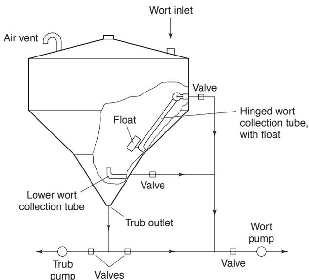
**Fig. 10.20** An empty hot wort settling tank (after Rehberger and Luther, 1994). After a period of settling clear wort is drawn from the top, through the floating, hinged arm. At the end of the settling period the last of the clear wort is collected from the lower collection point and then the trub, mixed with wort, is also drawn off.
