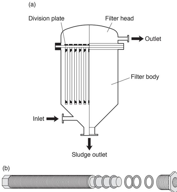
**Fig. 15.17** Candle filter or Metafilter; (a) candle filter, (b) detail of single candle (Hough *et al.*, 1982).
