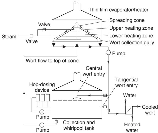
**Fig. 10.10** A diagram of a ‘Merlin’ wort boiling system in which the wort is collected in a whirlpool vessel and is heated, boiled and volatiles are stripped by pumping it in a thin film over a steam-heated cone in a separate vessel (after various sources, including Anton Steinecker literature).
