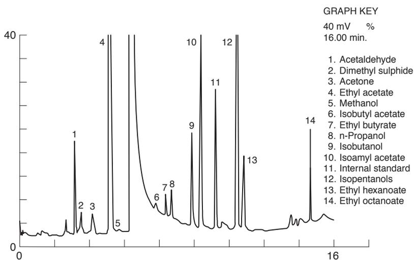
**Fig. 19.1** Typical chromatogram of volatile compounds in beer (Institute of Brewing, Methods of Analysis, 1997)
