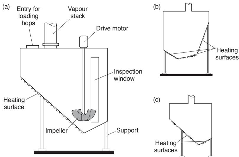
**Fig. 10.6** (a) A flat-sided, stainless steel copper (rectangular in plan) with an asymmetric heating surface of semicircular tubes, and an impeller to assist mixing the wort. This design maintained the same size of end wall, but provided vessels of differing capacity by altering the length of the vessel (after Hough *et al.*, 1982). (b) and (c) Cross-sections of alternative patterns of flat-sided kettles (after Rehberger and Luther, 1994).
