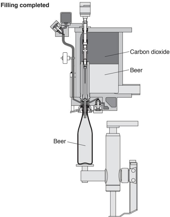
**Fig. 21.6** (f) Filling completed (beer in bottle) (by courtesy of Kronen).
