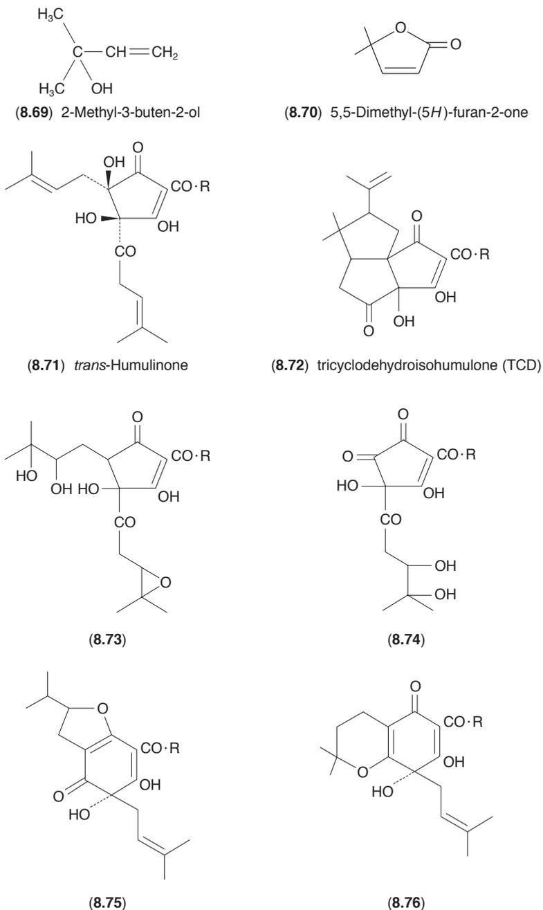
**Fig. 8.14** Oxidation products of the  $\alpha$ -acids.
