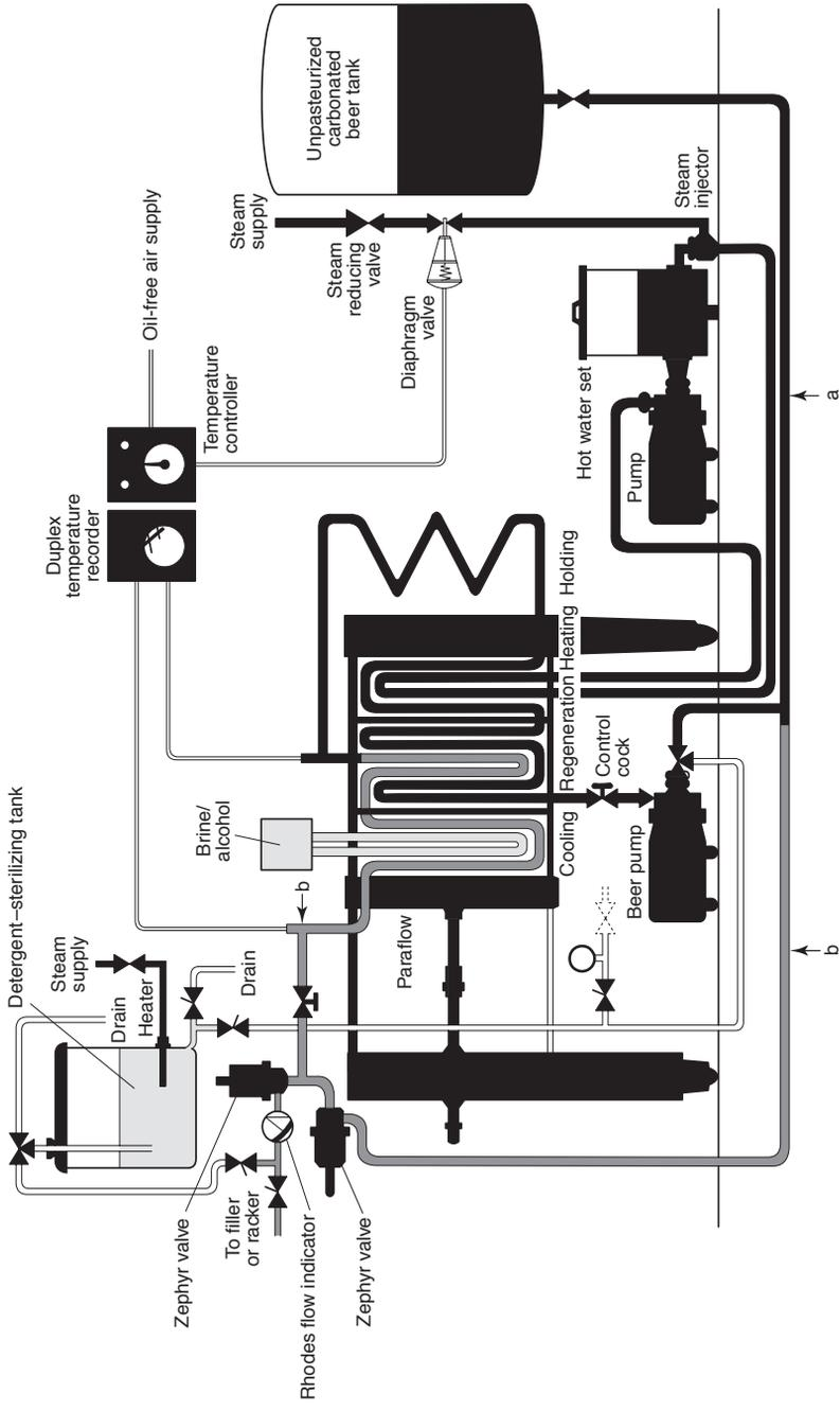
**Fig. 21.14** Flash pasteuriser; (a) raw unpasteurized beer, (b) pasteurized beer (by courtesy of APV Co. Ltd).
