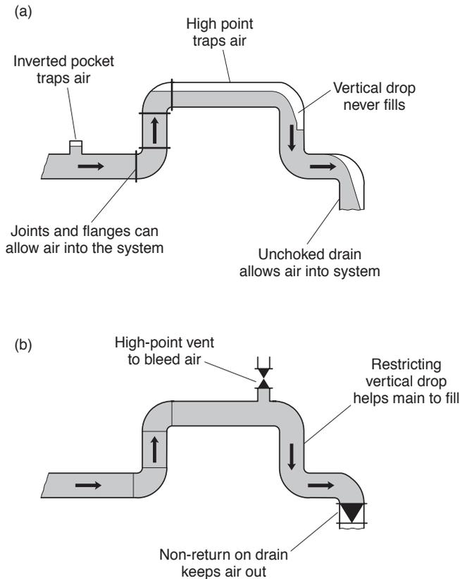
**Fig. 17.10** Poorly designed pipework (a) and some possible improvements (b) (Diagram courtesy of A. Mielenevski).
