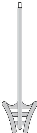
**Fig. 6.1** A wooden mashing rake or oar.
