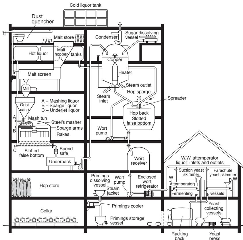
**Fig. 18.1** Sectional representation of a traditional small ale 'Tower' brewery, operating with one elevation of the wort to the Wort Boiler (Jeffrey, 1956).
