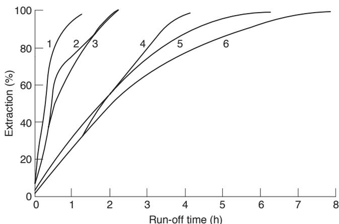
**Fig. 6.26** The patterns of the cumulative extract recovery against wort filtration time for various systems (Harris, 1968). (1) A Strainmaster lautering vessel. (2) A lauter tun loaded with a decoction mash. (3) A lauter tun loaded with a transferred infusion mash. (4) A mash tun with a medium depth of mash (1.52 m; 5 ft.). (5) A mash tun with a deep mash bed (2.44 m; 8 ft.). (6) A mash tun with a deep bed of grist containing both malt and maize grits, which slow wort separation.
