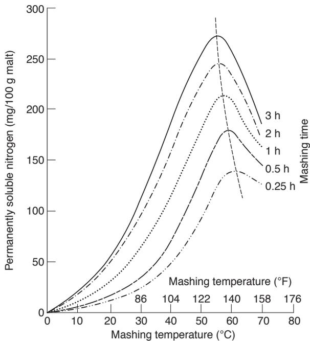
**Fig. 4.7** The influence of mashing time on the temperature optimum of the production of permanently soluble nitrogen (data of Windisch and Kolbach; after Moll *et al.*, 1974). With increasing incubation time the temperature 'optimum' declines (compare Fig. 4.1).
