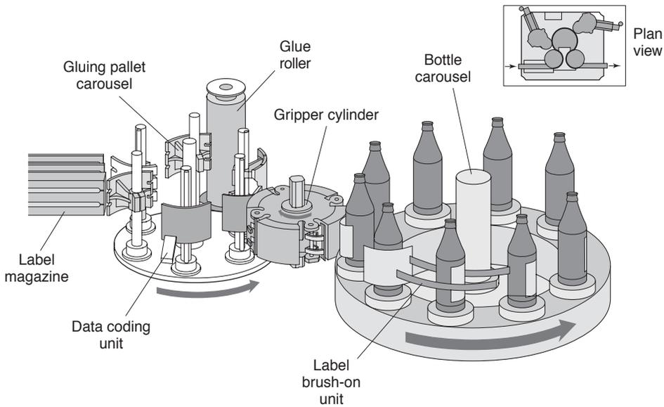
**Fig. 21.3** Bottle-labelling station (by courtesy of Krones).
