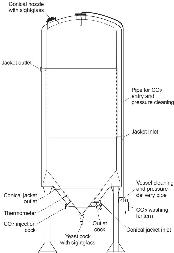
**Fig. 14.2** Cylindroconical fermentation vessel, (Hough *et al.*, 1982).
