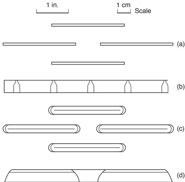
**Fig. 6.8** Slots in plates that form the false bottoms of mash tuns (after Briggs *et al.*, 1981). (a) Plan view of the upper surface. (b) Vertical section across the slots. (c) Plan view of the lower surface. (d) A vertical section, at right-angles to (b), along two slots.
